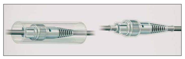
ZEUS Dual-Shrink® tubing of fluoropolymer PTFE/FEP is constructed with an exterior of heat shrink PTFE and an inner layer of FEP. It is easy to apply, and is designed to provide a tight, moisture-proof bond over wires, cables, connectors, splices, terminals, etc. The PTFE shrinks tightly over inserted parts when the covered section is heated, while the FEP melts and flows into a solid or near-
