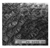
ePTFE with IND sizes ranging from  $1\mu$  to over  $200\mu$ .
