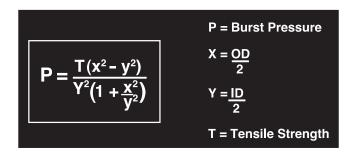
The above equation is theoretical. It does not factor steam pressure, altitude, etc., and it is calculated at ambient room temperature. The burst pressure result is meant as a guideline in design, not a definitive number.
