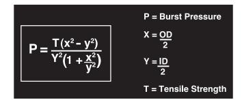
The above equation is theoretical. It does not factor steam pressure, altitude, etc., and it is calculated at ambient room temperature. The burst pressure result is meant as a guideline in design, not a definitive number.
